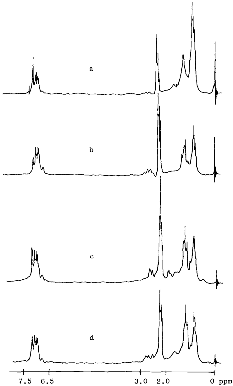
FIG. 2.—Nuclear magnetic resonance spectra of gasoline: (a) virgin; (b) weathered; (c) steam-distilled; (d) burned-steam-distilled.
